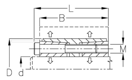
$\begin{array}{lll} \text{B mm} & = 80 \\ \text{d H8 mm} & = 75 \\ \text{D mm} & = 115 \\ \text{Fit tolerance} & = \text{Aksel h8, Nav H8} \\ \text{F kN torque} & = 179.0 \\ \text{L mm} & = 90 \\ \text{M mm} & = \text{M10} \\ \text{P N/mm2 surface pressure on shaft/hub} = 35 \end{array}$
